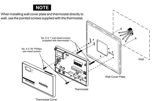
Figure 9. Mounting 1F60 thermostat to wall
